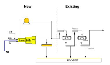
In the future, when greater capacity would be required, a recycle blower would be added to take the effluent vapor from the #1 sulfur condenser, and route it back to the reaction furnace, using sensible heat to carry away the heat of reaction. In essence, for oxygen operation, the recycle gas replaces the nitrogen normally entering with air under normal air operation.
