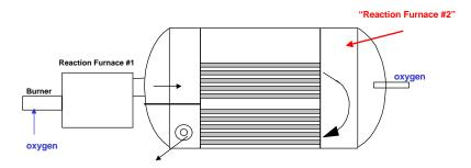
The first pass is the #1 WHB, the second pass is the #2 WHB, and the turn around space is used as the #2 reaction furnace. Thus for very little additional cost to normal replacement of the WHB the plant could be configured to take advantage of high concentrations of oxygen right from the start.
