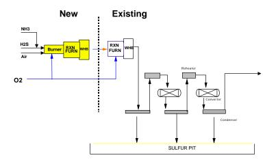
In the first reaction furnace, all amine acid gas, all sour water stripper gas (if any), and all air are fed to the new BOC burner. Only oxygen is split between the first and second
