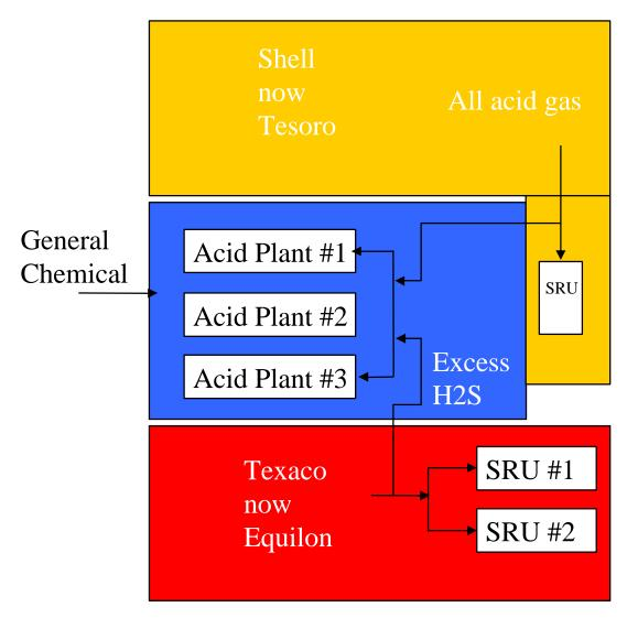
The sulfur plant first owned by Shell Anacortes Refining Company and now owned by Tesoro Northwest Company is located adjacent to General's sulfuric acid plants. All of the amine acid gas from the refinery once owned by Shell is sent to General. Some is processed in the SRU owned by the refinery and operated by General. The remainder is used as fuel in the sulfuric acid plants.
